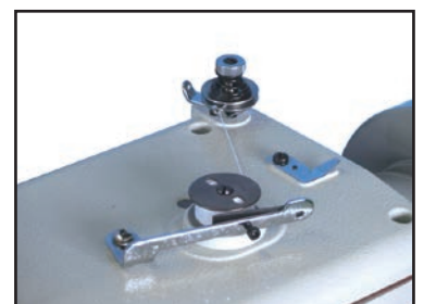
Built-in bobbin winder that enables simple and fine adjustment of winding volume of threads
