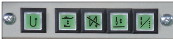
Simple setting for alternating presser foot movement
