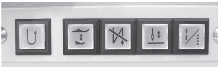
Simple setting for alternating presser foot movement
