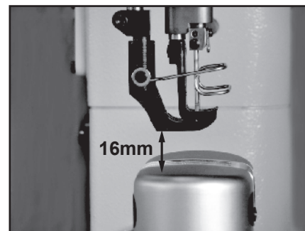
The clearance under the presser foot (16mm)
