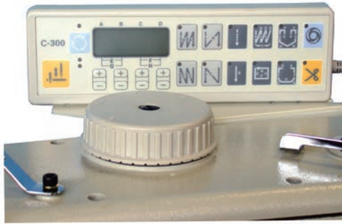
Simple setting for walking foot movement
