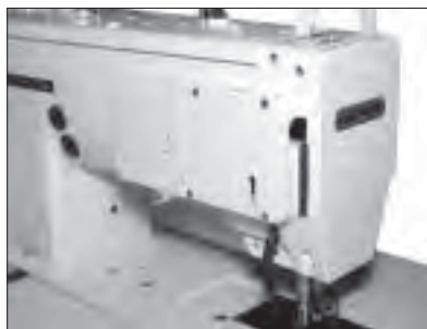
Open/close simplified face plate and upper feed mechanism
