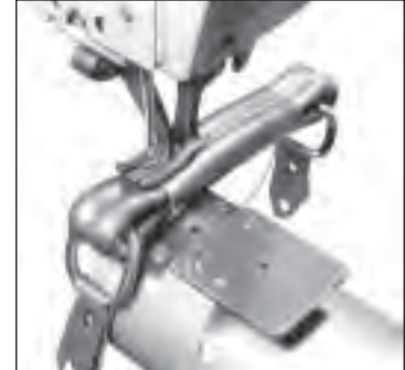
Sewing heavy thick bag handle by CH-8B of special specifications
