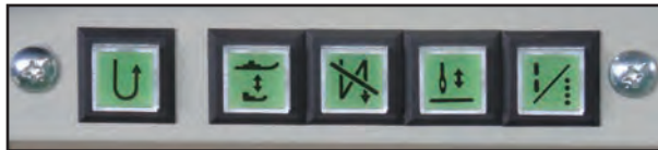
Simple setting for alternating presser foot movement
