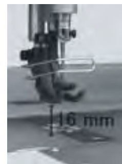
The clearance under the presser foot (16mm)
