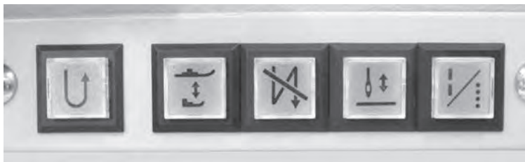
Simple setting for alternating presser foot movement
