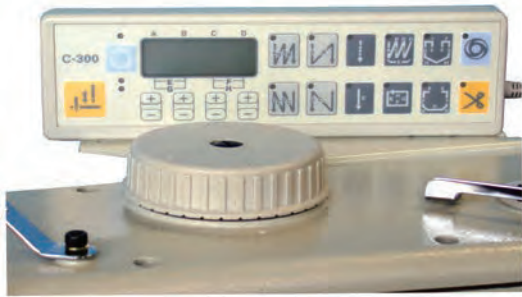
Simple setting for alternating presser foot movement
